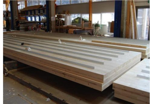
Plywood boards with HBV®-Shear Connector
