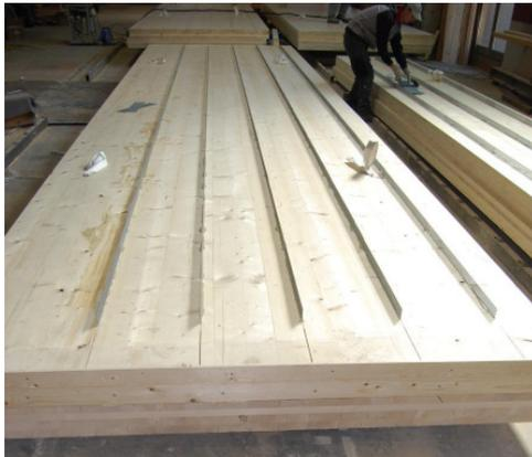
Plywood boards with HBV®-Shear Connector
